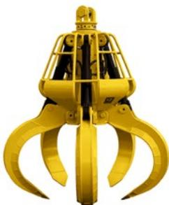
Its robust design makes it suitable for handling rough scrap metal and for the harsh conditions in scrap yards, waste sites, or in quarries. The independently driven separate jaws and high-quality hydraulic rotator ensure that a load of any shape may be grabbed. Possibility to supply with hydraulic forced swivelling (standard), with mechanical swivelling or with a fixed hinge for the grab.
